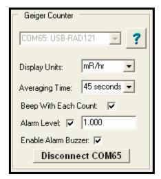
This area allows you to connect to and configure the Geiger counter attached to your computer. The drop down lets you select which device you'd like to connect to.
