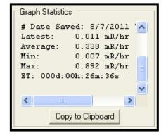
This area shows you statistics for the graph, including the latest sample time, average reading, minimum and maximums, and elapsed time.
